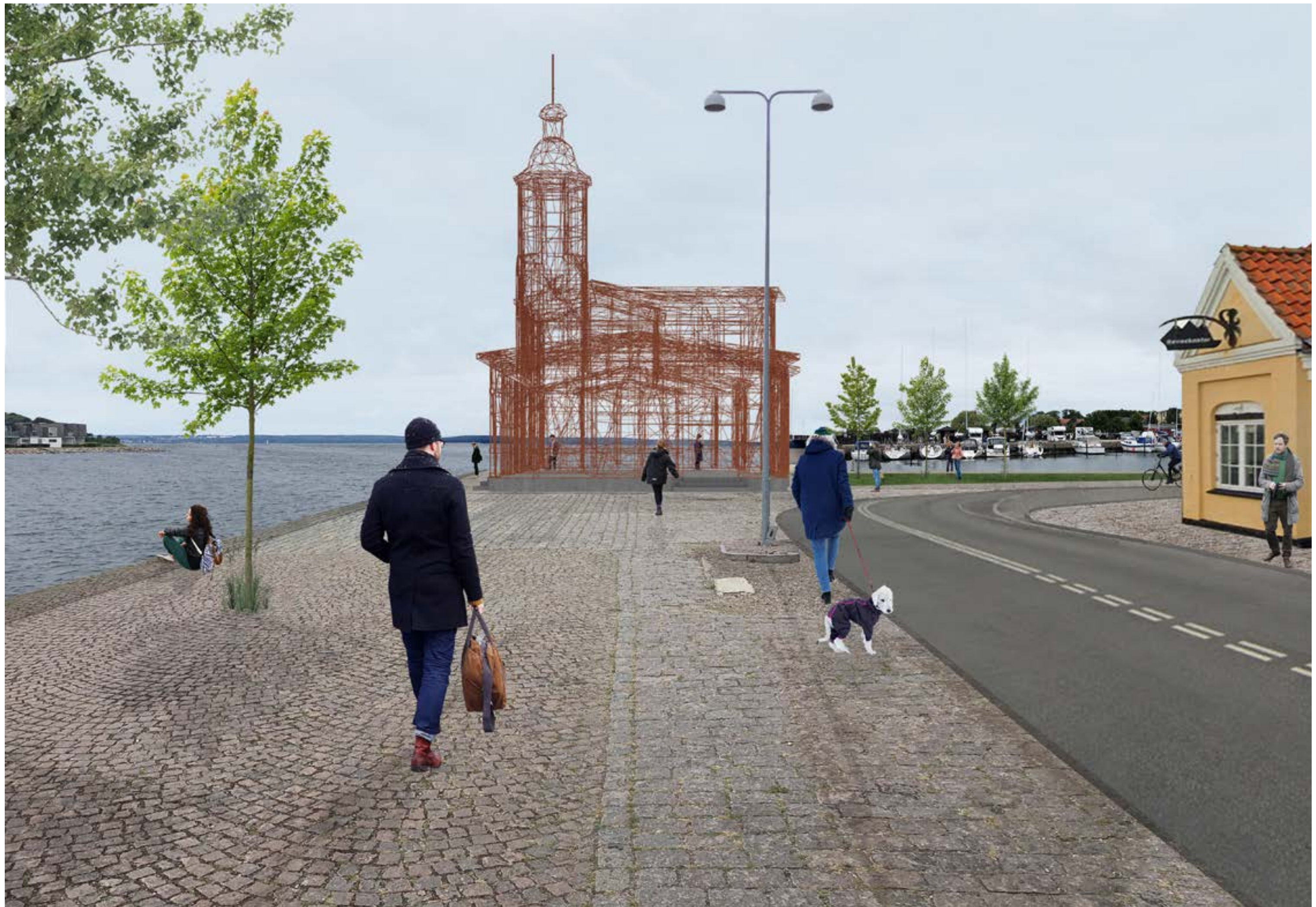
Optimised triangulated mesh, 38,5 tonnes, perspective view
